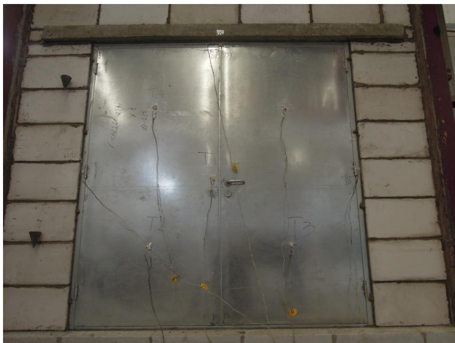
Fig. 2 – Unexposed Side Prior to the Fire Test
