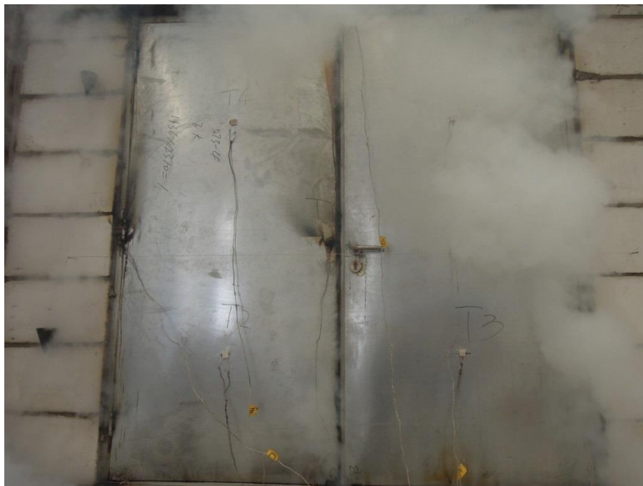
Fig. 4 – Unexposed Side after 40 Minutes
