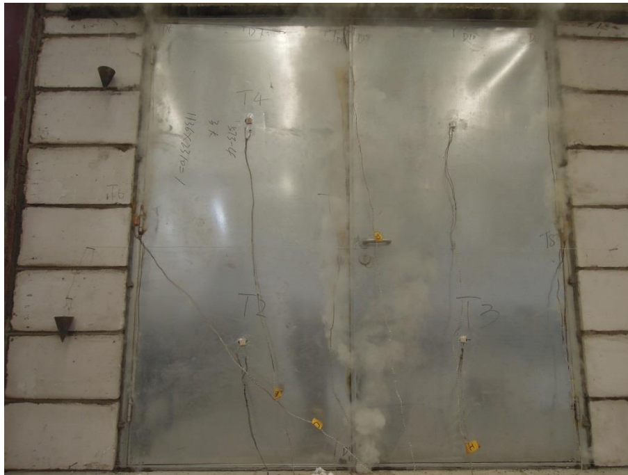
Fig. 3 – Unexposed Side after 20 Minutes
