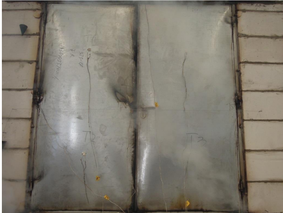
Fig. 5 – Unexposed Side after 60 Minutes
