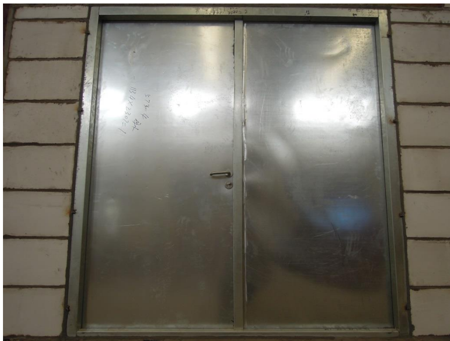
Fig. 1 – Exposed Side Prior to the Fire Test
